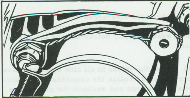
Figure 5-56 Intake Pipe at Cylinder
